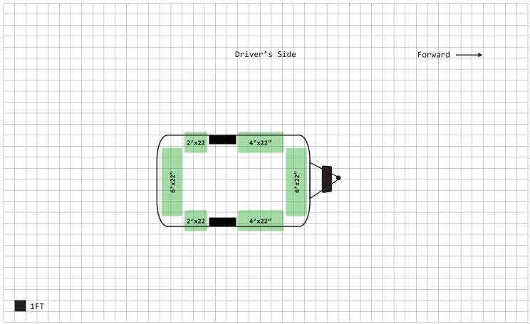
Suggested configuration - tubes may be positioned in alternative configurations Tube overlap and gaps on diagram possible due to tube compression, bend, and elasticity Stair, slide, and tire positioning are approximate Tubes conform around objects such as stairs and drain pipes Airstream Travel Trailer 16 Feet support@airskirts.com 833.475.4787
