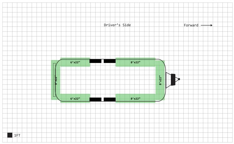
Suggested configuration - tubes may be positioned in alternative configurations Tube overlap and gaps on diagram possible due to tube compression, bend, and elasticity Stair, slide, and tire positioning are approximate Tubes conform around objects such as stairs and drain pipes
