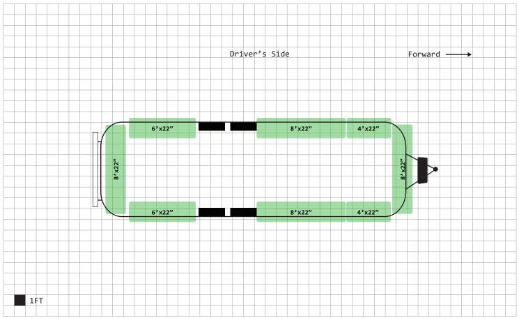
Suggested configuration - tubes may be positioned in alternative configurations Tube overlap and gaps on diagram possible due to tube compression, bend, and elasticity Stair, slide, and tire positioning are approximate Tubes conform around objects such as stairs and drain pipes Airstream Travel Trailer 30 Feet support@airskirts.com 833.475.4787
